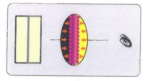
> If one pass is not enough, repeat the operation on the right and on the left of the first pass until the panel returns to its original shape.
