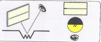
As with all deep dents, the board must be very close to the dent in order to see its bottom. Start pushing and lifting the centre of the dent so that the jagged bottom surface of the dent appears.
