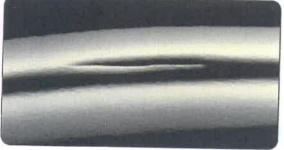
Small 10 cm crease with a slightly creased bottom. To fix this, we'll use a round stainless steel tip.
