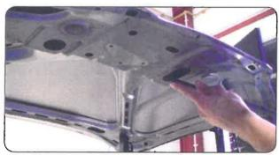
Direct access through a hole in the brace. Be careful not to deform the inner panels.
