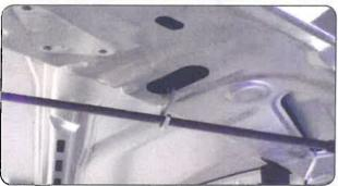
Hook used hanging from a hole in the inner panel or brace.
