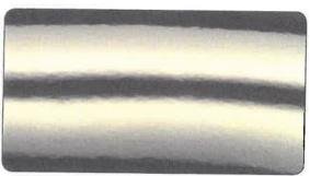
Once the high spot is tapped down, the panel should be in its original shape. The black line and fog are now identical to an unaffected area of the panel. The dent is repaired.
