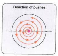
The same pressure must be applied for each push. The pushes must be connected together so that the orange peel isn't affected. The last quarter of the dent will pop out automatically.
