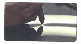
The dent has been pushed up at the centre and now has a high spot. Next, check the height of each dent closely during the final stage of its repair (until original shape is reached). The high spot must be tapped down to make it level.
