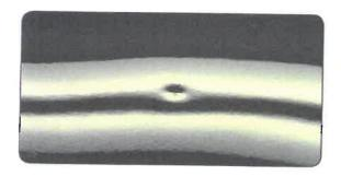
The jagged impression appears in the form of a star, so each line that forms the star must be pushed. The board must be placed parallel to each line.
