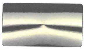
The dent must be pushed up to create a high spot in order to eliminate the point of impact.
