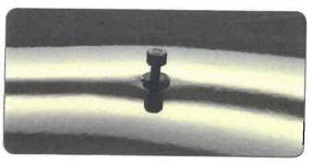
Position the glue tab on the centre of the dent. The glue tab must be smaller than the dent since it needs to lift up the bottom of the dent.
