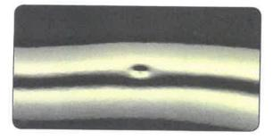
Small and deep sharp dent. To fix this, we'll use a pointed stainless steel tip.
