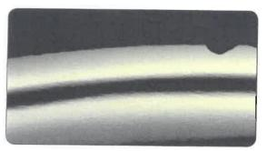
When the crease is repaired, the black line and the fog must be identical whether in the area of deformation or not.
