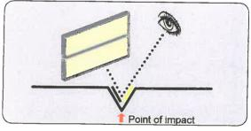
Proper Board position. Board close in order to see the bottom of the dent.
