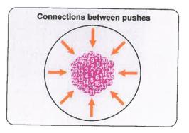
This step sometimes must be repeated several times depending on the depth of the dent. You must alternate your position with each pass: one from the front, one from side and so forth. Gradually move your board away between passes until the panel returns to its original shape (height of dent).
