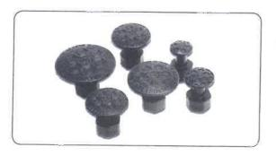
The pulling tools use hard plastic glue tabs with diameters between 12 mm and 32 mm. These glue tabs are shaped to provide maximum hold with the hot glue used for pulling out the dent. This glue is specifically designed to be used for dent removal. Different hot glues exist with varying degrees of adherence depending on the working temperature.
