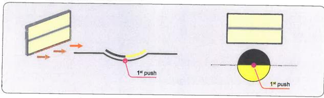
Position the Board so that you obtain a half yellow/half black line. This will indicate the centre of the dent in a vertical direction; you will then have to centre it yourself in the horizontal direction. Begin to push lightly to see how your dent reacts. You are in the centre of the dent when all the edges of the dent pull towards the centre.
