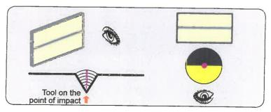
Position the tool precisely under the point of impact and begin pushing around lightly and playing with the elasticity, relieving the pressure when an outward dent is about to form (up to the elastic limit).
