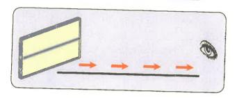
The light is diffused, the black line remains straight and the fog is the same from left to right. No impact exists.
