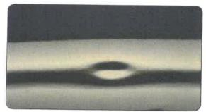
Smooth dent with plenty of elasticity and a rounded bottom.
