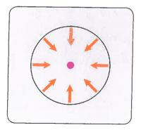
Do the 1<sup>st</sup> push, and then proceed in a circle around this point. Continue the spiral pattern in a counterclockwise direction for ¾ of the dent.
