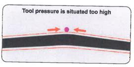
The indentation doesn't appear yet; the line is bowed too high. The tool is too high (the fog remains the same).
